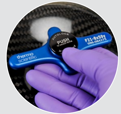
Auto-Lock rotor exchange
